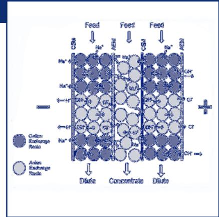
In traditional ion exchange units, after the contaminants are trapped onto the resin sites, the resin continues to exhaust and lose capacity. In EDI, the contaminants are continuously removed as they are attracted to one of the two electrical charges, and then migrate through the resin bed, through ion exchange membranes and into the concentrate stream where they are removed from the device.
