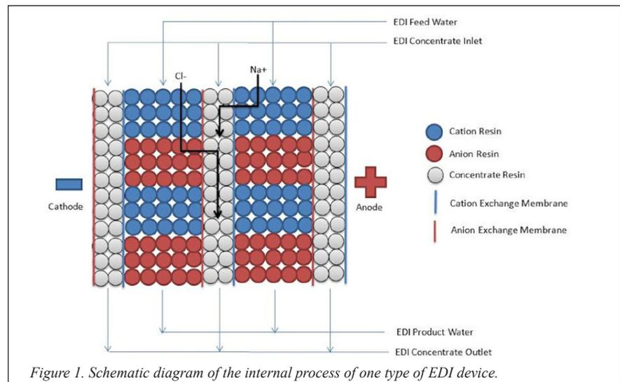
Figure 1. Schematic diagram of the internal process of one type of EDI device.
